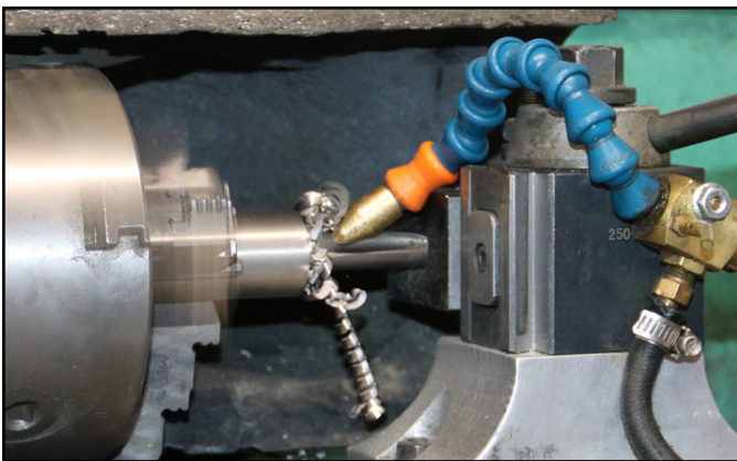
The engraver removing excess titanium to shape the ring to the precise shape.
