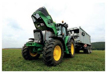
In 2017, John Deere showcased the first, fully battery-powered tractor. This technological innovation is truly the first of its kind. Nicknamed SESAM, for Sustainable Energy Supply for Agricultural Machinery, this all-electric tractor is modeled after John Deere's 6R Series Tractors.
