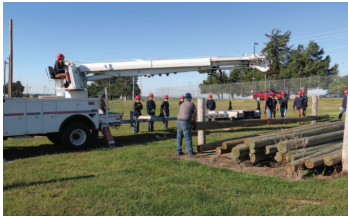
Brittany Grammer uses one of Northeast Community College's trucks to load electric power poles onto a waiting trailer.
